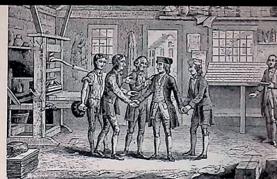
Above ● Here is an artist's idea of how the printing plant of Benjamin Franklin appeared. At the right can be seen the cases which hold the pieces of metal type. At the left appears the old-fashioned printing press which was laboriously run by a strong-armed pressman.
